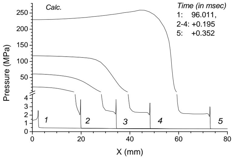
Fig. 2. Computation of explosion development in the wetted AN+DCCNa mixture with reduced ignition temperature of the mixture. Evolution in time of the pressure profile.
