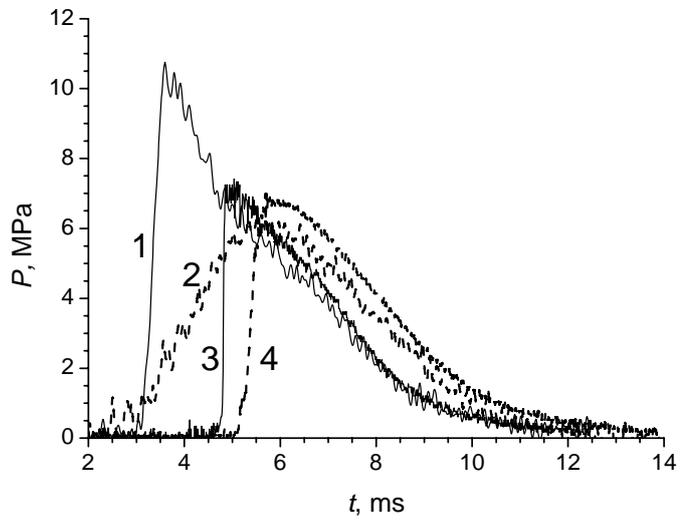
Fig. 1. Pressure–time profiles recorded at two points along the charge at a distance 40 and 145 mm from the closed charge end in two tests with the dry (curves 2 and 4) and wetted (curves 1 and 3) mixtures initiated by the igniter-cap.
